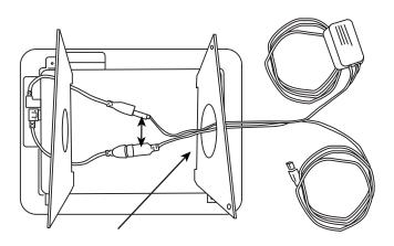
Remove the four small screws from the camera tower located along the rear edge above the center camera location. Use four of the longer screws included with the tablet accessories to attach the tablet assembly to the camera tower
